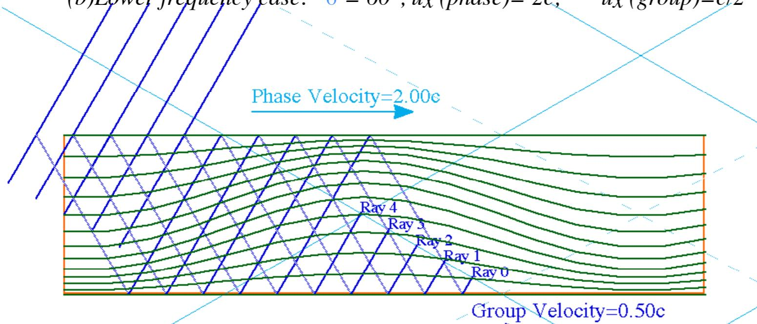
$$u_x(\text{phase}) = \omega/k_x = c\omega / \sqrt{(\omega^2 - \pi^2 c^2/W^2)}$$
