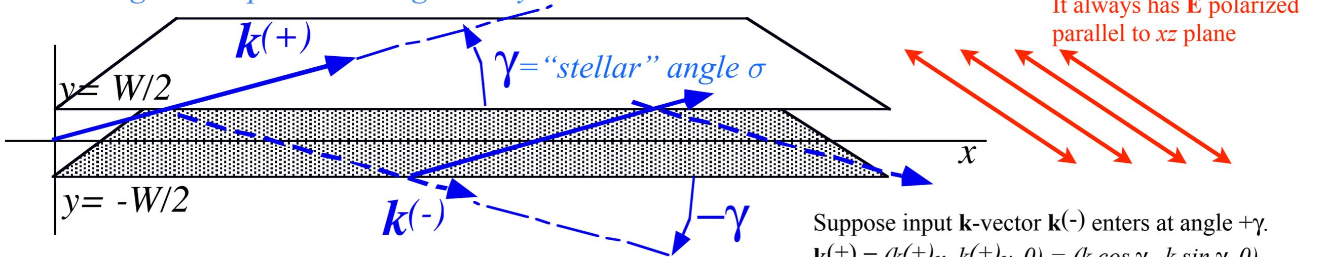
Fig. 6.3.1 "Hall of mirrors" model for an optical wave guide of width W.
