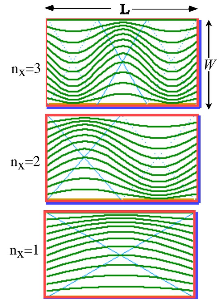
Fig. 6.3.7 Cavity modes for three lowest quantum numbers
