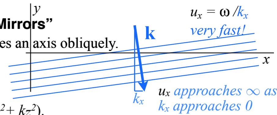
Consider 'Hall of Mirrors' with two parallel mirrors on either side of the  $x$ -axis be separated by a distance  $y=W$ . The South wall will be at  $y=-W/2$  and the North wall at  $y=W/2$ . ( $z$ -axis or "up" is into the page here.) The Hall should have a floor and ceiling at  $z=\pm H/2$  as discussed later. Here waves move in  $xy$ -plane only.
