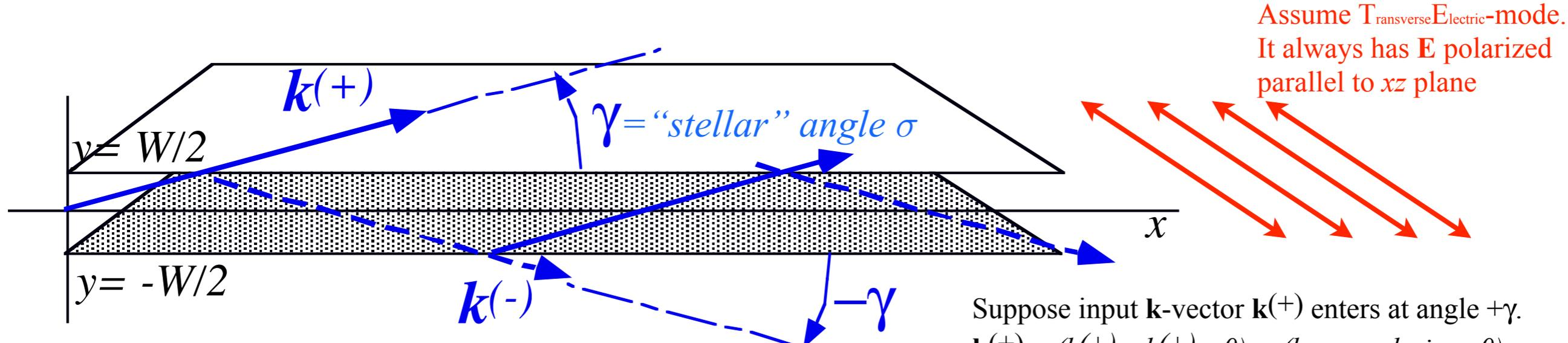
Fig. 6.3.1 "Hall of mirrors" model for an optical wave guide of width  $W$ .
