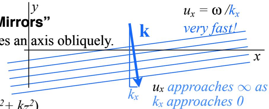
Consider 'Hall of Mirrors' with two parallel mirrors on either side of the  $x$ -axis be separated by a distance  $y=W$ .
