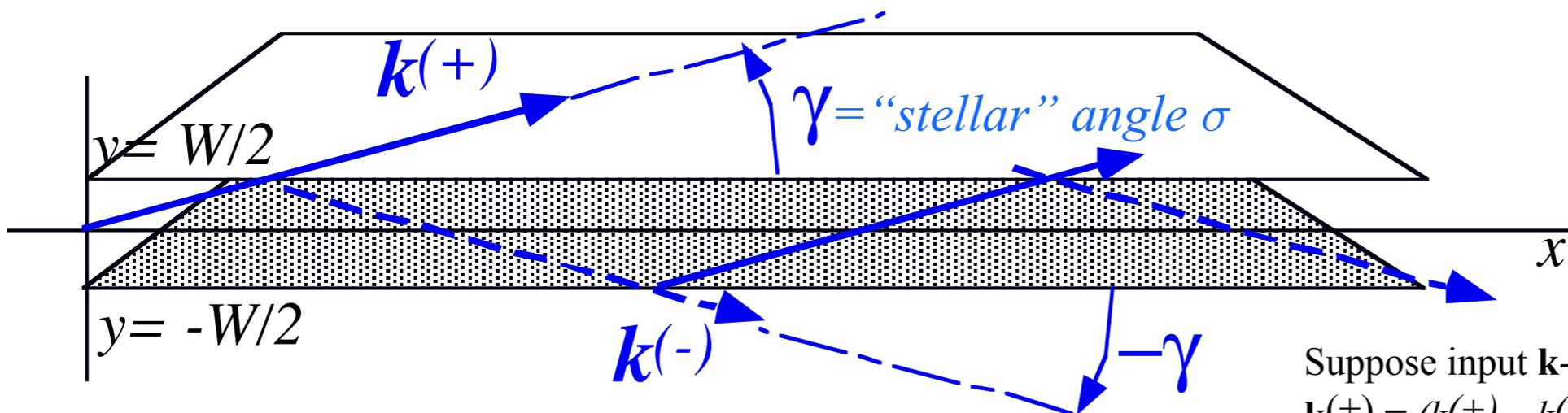
Fig. 6.3.1 "Hall of mirrors" model for an optical wave guide of width  $W$ .
