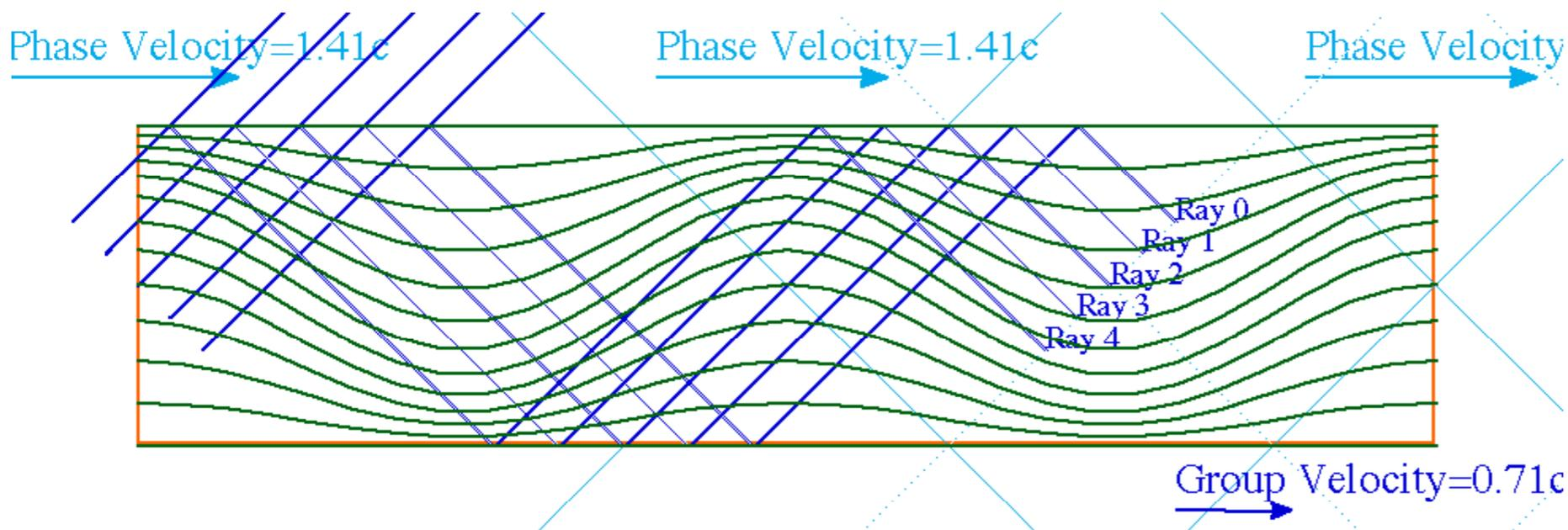
Fig. 6.3.4 Right moving guide wave with  $\sigma = 45^\circ$ ,  $V_{phase}=\sqrt{2}c$ ,  $V_{group}=c/\sqrt{2}$ .
