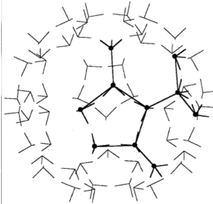
Fig.8 60 orthonormal triads of coordinate axes. Unit cell used to define force matrix has thicker lines
