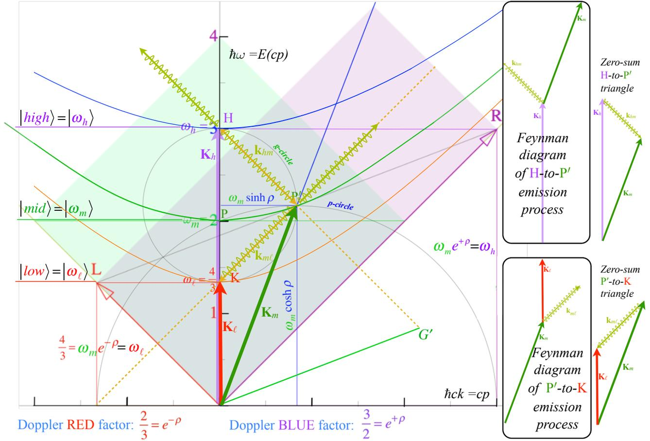
Fig. 19 Feynman diagrams of 1-photon transitions connecting 3-levels  $\omega_h$ ,  $\omega_m$ , and  $\omega_\ell$ .
