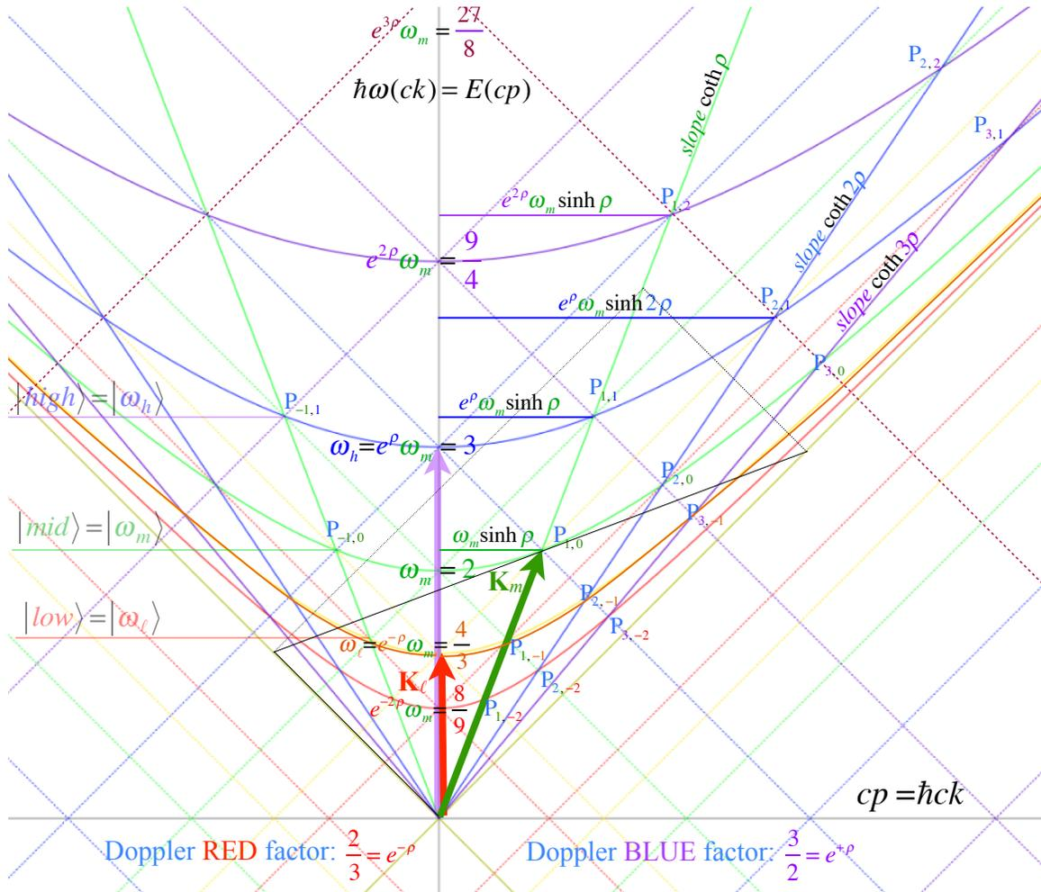
Fig. 20. Rapidity- $\rho_p=p\rho$  and rest-frequency- $\omega_m e^{q\rho}$  and  $P_{p,q}$ -lattice based on integer powers of  $b=e^{\rho}=\frac{3}{2}$ .
