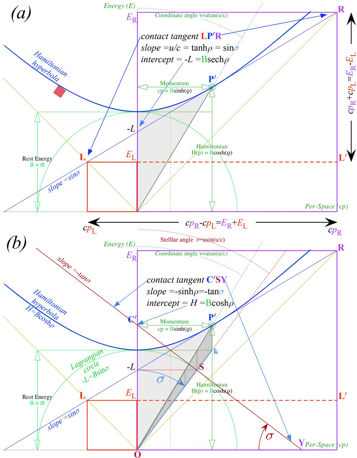
Fig. 14 Legendre transform: (a) Slope  $u/c$  and intercept  $-L$  of  $H(p)$ -tangent  $LP'$  give  $(u, L)$  point  $S$  on  $L(u)$ -circle. (b) Slope  $cp$  and intercept  $H$  of  $L(u)$ -tangent  $C'S$  give  $(p, H)$  point  $P'$  on  $H(p)$ -hyperbola.
