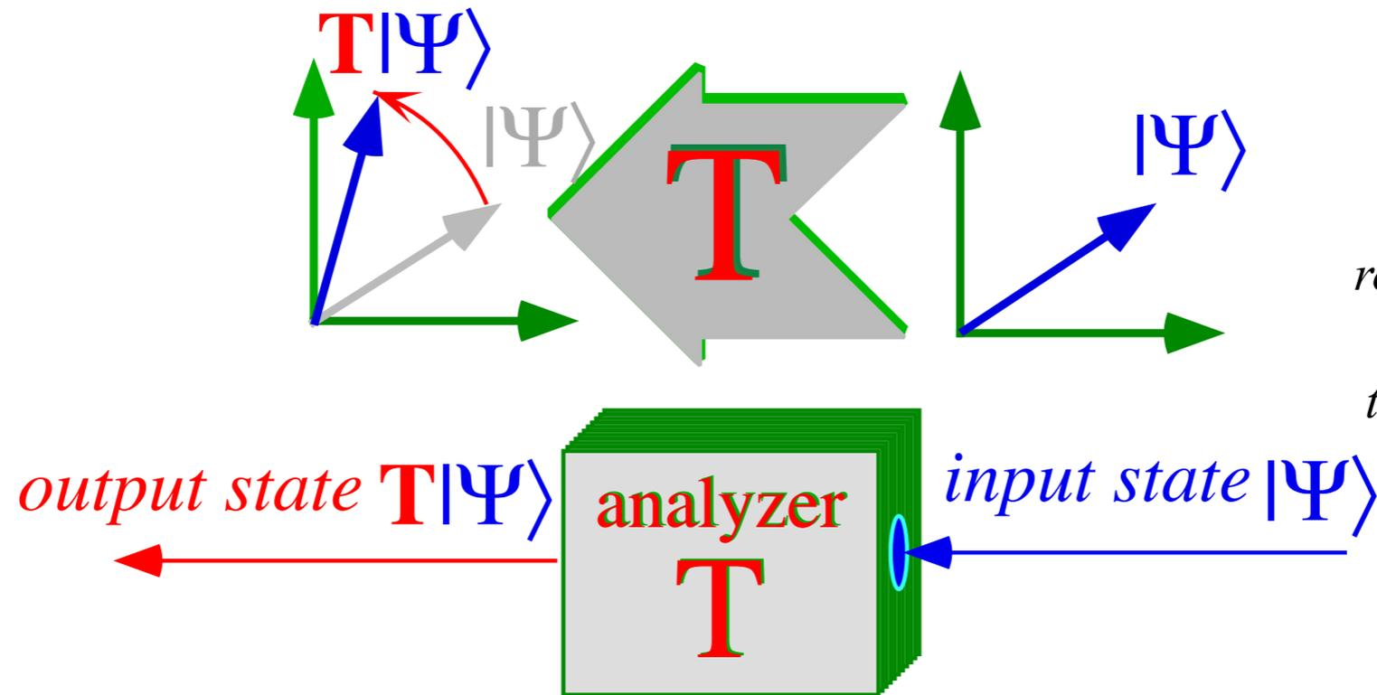
Fig. 3.1.1 Effect of analyzer represented by ket vector transformation of  $|\Psi\rangle$  to new ket vector  $T|\Psi\rangle$ .
