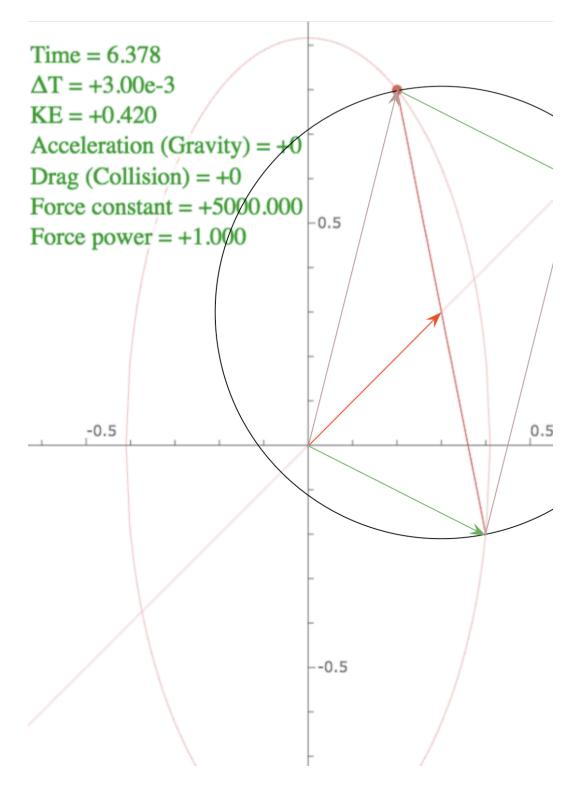
Example with  $(V^{IN_1}, V^{IN_2}) = (0.4, +0.2)$ . Final velocities are closer so elastic and inelastic ellipses nearly overlap. The 45° Galilean lines are tangent to a much smaller COM ellipse.
