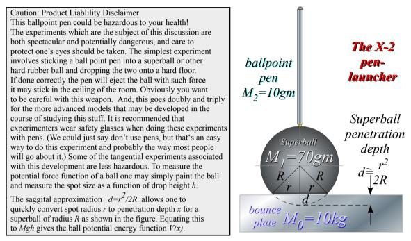
Fig. 4.1 The X2-pen launcher with product liability disclaimer.
