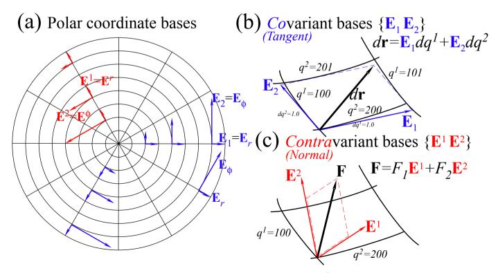
Fig. 12.10 Covariant force vector components in a polar space ( $\mathbf{E}^{\rho}, \mathbf{E}^{\phi}$ ).
