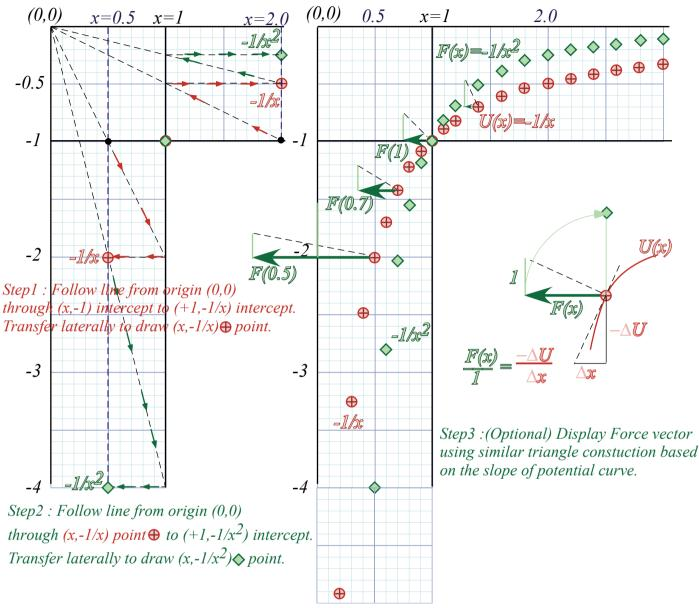
Fig. 9.5 Attractive Coulomb force F(x) and potential U(x) curves. ( $\mathbf{F}(x)$  vectors drawn at 1/4-scale.)
