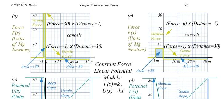
Fig. 7.3 Force and potential plots. (a-b) Strong (30g) deceleration. (c-d) Medium (6g) deceleration.
