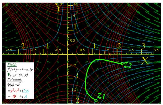
$$Kajobian = \begin{pmatrix} \frac{\partial q^{1}}{\partial x} & \frac{\partial q^{1}}{\partial y} \\ \frac{\partial q^{2}}{\partial x} & \frac{\partial q^{2}}{\partial y} \end{pmatrix} = \begin{pmatrix} \frac{\partial \Phi}{\partial x} & \frac{\partial \Phi}{\partial y} \\ \frac{\partial A}{\partial x} & \frac{\partial A}{\partial y} \end{pmatrix} = \begin{pmatrix} x & -y \\ y & x \end{pmatrix} \leftarrow \mathbf{E}^{\Phi}$$
