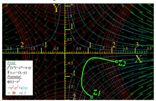
$$Metric tensor = \begin{pmatrix} g_{\Phi\Phi} & g_{\Phi A} \\ g_{A\Phi} & g_{AA} \end{pmatrix} = \begin{pmatrix} \mathbf{E}_{\Phi} \cdot \mathbf{E}_{\Phi} & \mathbf{E}_{\Phi} \cdot \mathbf{E}_{A} \\ \mathbf{E}_{A} \cdot \mathbf{E}_{\Phi} & \mathbf{E}_{A} \cdot \mathbf{E}_{A} \end{pmatrix} = \begin{pmatrix} r^{2} & 0 \\ 0 & r^{2} \end{pmatrix} \text{ where: } r^{2} = x^{2} + y^{2}$$
