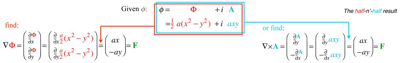
Scalar static potential lines  $\Phi$ =const. and vector flux potential lines  $\mathbf{A}$ =const. define DFL field-net.
