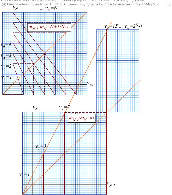
1<sup>st</sup> case shows *linear* series of final velocity. 2<sup>nd</sup> case shows *geometric* or *exponential* series of velocity.
