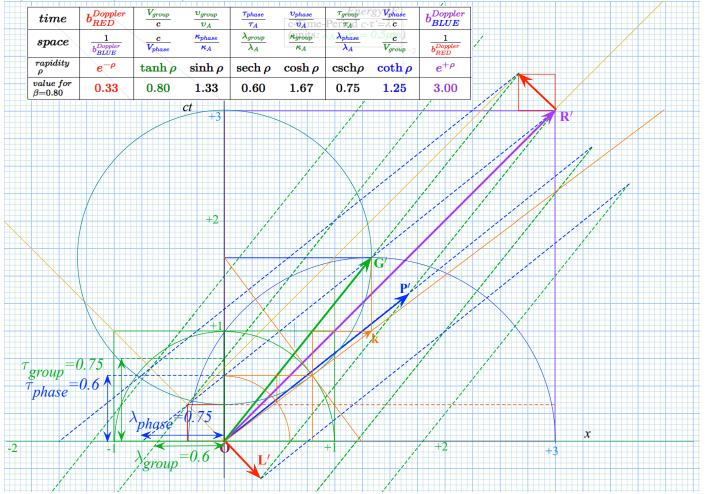
This space-time plot has the base circle rescaled to unit radius so the dimensionless wavelengths and periods have the values listed in the tables shown correctly on the graph.
