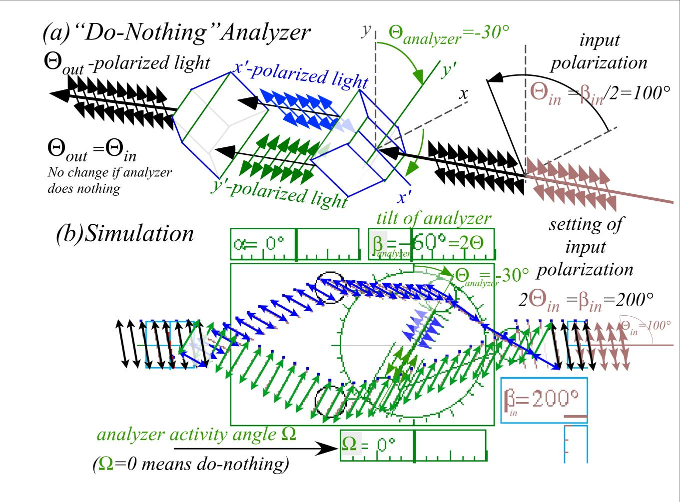
Imagine final xy-sorter analyzes output beam into x and y-components.
