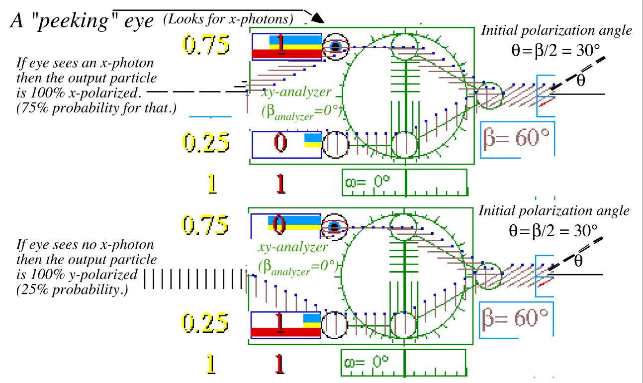
Fig. 1.3.7 Simulated polarization analyzer set up to "peek" if the photon is x-or y-polarized
