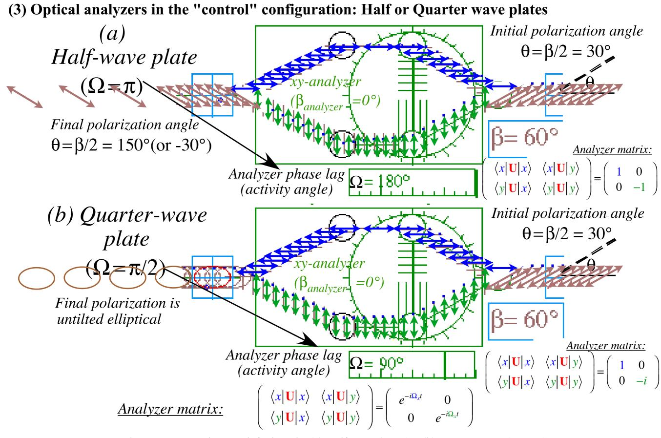
Fig. 1.3.5 Polarization control set to shift phase by (a) Half-wave ( $\Omega = \pi$ ), (b) Quarter wave ( $\Omega = \pi/2$ )
