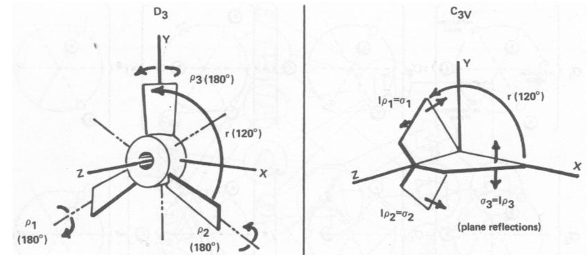
**Figure 3.1.3** Pictorial comparison of  $D_3$  and  $C_{3v}$  symmetry. A propeller having  $D_3$  symmetry is shown next to a three-plane paddle having  $C_{3v}$  symmetry. The group operations are labeled by arrows, which indicate the effect they have. For example,  $\rho_3$  is a 180° rotation around the y axis, while  $I\rho_3 = \sigma_3$  is a reflection through the xz plane. (Here axes are fixed and the objects rotate.)
