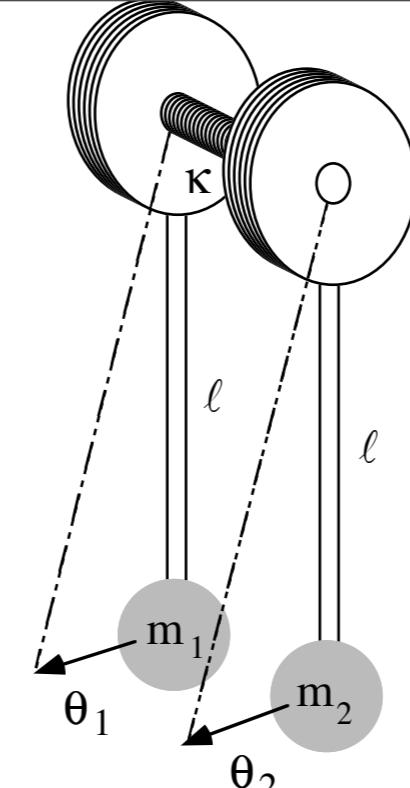
Fig. 3.3.2 Coupled pendulums
